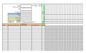
By combining the concept diagram and the master plan, the lock plan is created – the entire system. Planning and ordering masterkey systems is fairly simple. The process is shown in the sample plan below. All the doors are listed horizontally; the vertical columns are for the keys. More information about planning of masterkey systems can be obtained at KESO training courses or from your specialist.
